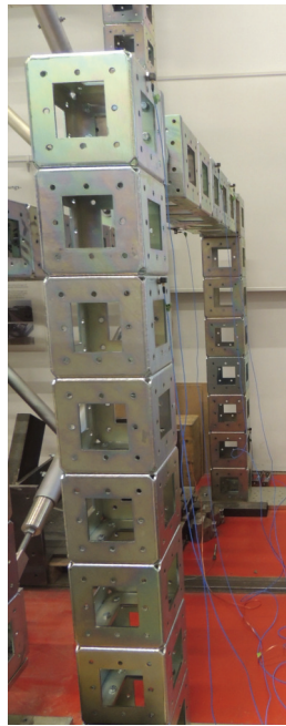
(a) Studied structure constructed from steel cubes
