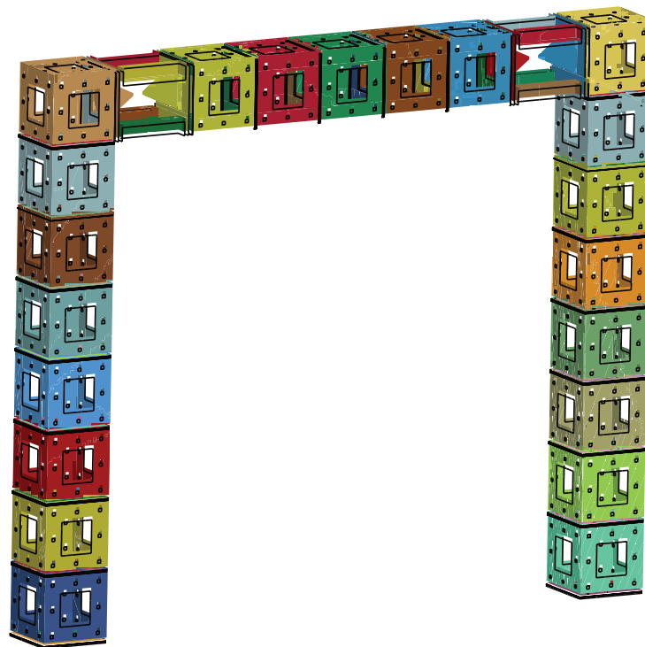
Figure 5.14: Numerical model of the studied frame using shell elements
